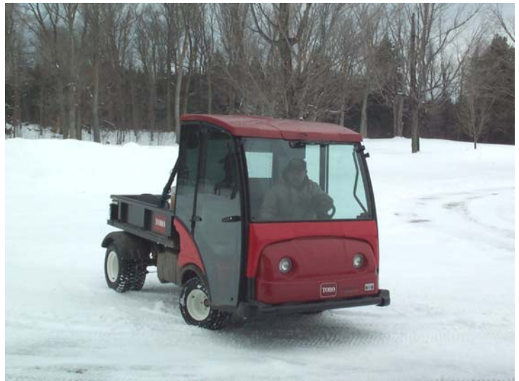
The new Toro Workman has a Kubota diesel engine, 4-wheel drive and a heated cab for year round work..
